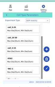
Figure 10-36 Cell Parameter Settings
