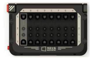
Note 1: If you have fewer than 8 samples, fill empty slots with Chip P (no reagents are added to Chip P).
