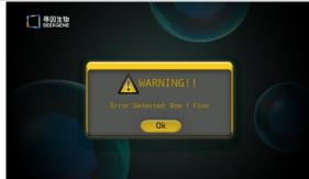
Please check if the sealing gasket is clean, if the chip has any damage on its surface, and if the Chip Holder is installed correctly. If there is dirt in the sealing gasket or damage on the chip's surface, please replace the gasket or chip and try again. If the error message recurs, contact (info@seekgene.com) for further assistance.
