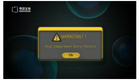
The operation in and out of the warehouse may be blocked. Please confirm that no objects are blocking the running path and click the "OK" button on the prompt window. The instrument will proceed to the next step. If the message appears repeatedly, please contact (info@seekgene.com) for further assistance.
