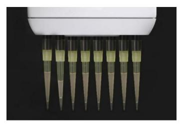
**Note**: If the solution is like in the second tip from the left in the figure, it indicates a clog.
