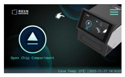
2. Put the Chip Holder with the covering Gasket into the tray according to the illustration, make sure the Chip Holder is placed horizontally, and click the "Close Chip Compartment" button to retract the fixture tray.
