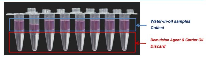
**Note 1**: The resulting mixture (shown above) includes Demulsion Agent/Carrier Oil (clear) and aqueous phase reaction solution (pink).
