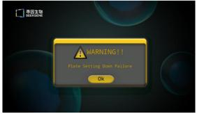
Please verify if the gasket is properly seated on the Chip Holder and reposition the Chip Holder. Check if there are any foreign objects on the surface of the chip compartment and clean the surface. If the message appears repeatedly, please contact (info@seekgene.com) for further assistance.
