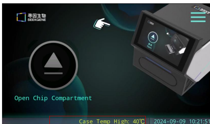
Figure 8-3 Case Temperature Too High
