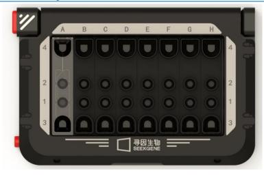
**Note 1**: If there are less than 8 samples, the empty chip positions must be replaced with Chip P. The 8 chip positions in the chip holder should not be left empty. **But nothing is pipetted into Chip P!**
