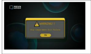
The operation in and out of the warehouse may be blocked. Please confirm that no objects are blocking the running path and click the "OK" button on the prompt window. The instrument will proceed to the next step. If the message appears repeatedly, please contact (info@seekgene.com) for further assistance.
