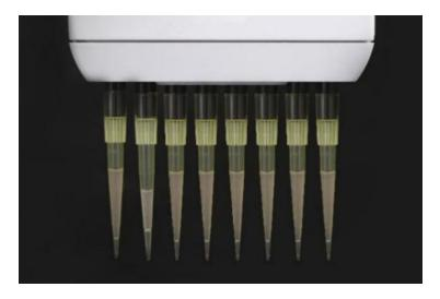
**Note**: If the solution is like in the second tip from the left in the figure, it indicates a clog.
