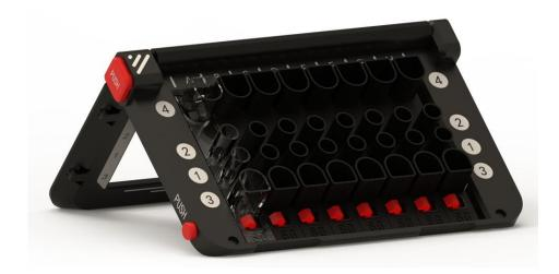
3. Check Wells 1 and 2: Inspect Wells 1 (aqueous phase) and 2 (adhesive bead phase). Any unusually high volume indicates a clog.
