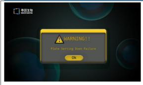
Please verify if the gasket is properly seated on the Chip Holder and reposition the Chip Holder. Check if there are any foreign objects on the surface of the chip compartment and clean the surface. If the message appears repeatedly, please contact (info@seekgene.com) for further assistance.
