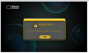
Please check if the sealing gasket is clean, if the chip has any damage on its surface, and if the Chip Holder is installed correctly. If there is dirt in the sealing gasket or damage on the chip's surface, please replace the gasket or chip and try again. If the error message recurs, contact (info@seekgene.com) for further assistance.
