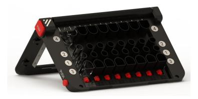
3. Check the volume of the single-cell mixture and Barcoded Beads solution in both Well 1 and Well 2. Abnormally high volume in either well indicates a clog.
